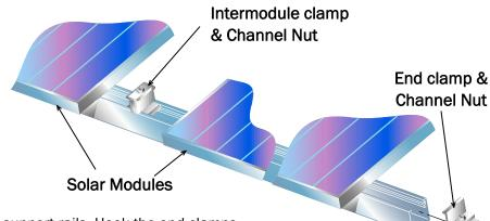
Insert an end clamp at the end of each row of support rails. Hook the end clamps against the long end of the module and square off to the support rail. Tighten the clamps using a 1/2" box wrench or drive socket. DO NOT OVER-TIGHTEN, we recommend a maximum torque of 12-15 ft. lbs. to prevent damage to the module glass.
