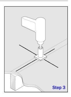
STEP 3: Using a cordless impact wrench and a 9/16" deep socket, install the bolt into the SolarWedge® base until seated. Allow the sealant to flow outward around the edges of the seal plate.
