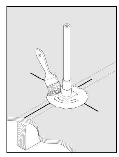
STEP 5: Seal the top of the seal plate with a layer of UV rated seal-ant using a stiff paintbrush. Cover the entire base plate with the seal-ant, at least half the post and about 1-1/2" around the plate.
