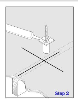
STEP 2: Apply a generous amount of roof sealant to the bottom of the seal plate of the SolarWedge® creating a circle around the lag bolt hole.
