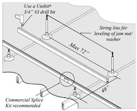
STEP 1: Using a string line from each end of the module array, level studs to desired position on roof (4" leveling stud must have at least 1" threaded into post).
