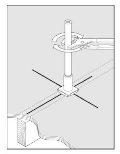
STEP 4: Install the post using an adjustable wrench. Turn wrench clockwise until fully secured. Avoid twisting the base while tightening.
