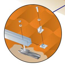
Illustrated above is bow the Tile Trac® attachment seamlessly integrates with the Roof Trac™ mounting system.
