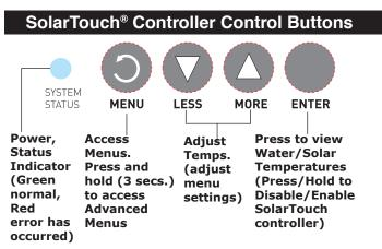
**Main Screen:** In normal operating mode the main screen displays the current WATER temperature, TARGET Temperature and if SOLAR HEAT, NOCTURNAL COOLING or FREEZE is ON or OFF. Press the Enter button to view the current Water and Solar temperatures. If no menu activity is detected after two minutes, the main screen is displayed.
